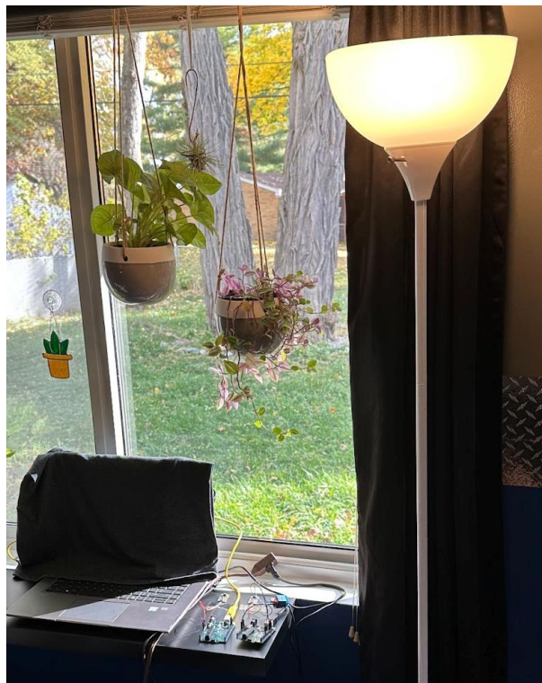
Figure 3.5-2: Daylighting Control System with Illuminance Sensor
